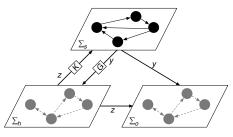
Networked system nodes y  $(\Sigma_s)$ , virtual nodes z  $(\Sigma_h)$ , observation nodes  $(\Sigma_o)$ :
