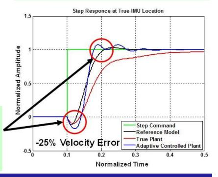
**Unmatched Uncertainty can Result in Oscillations in the True IMU Accel**
