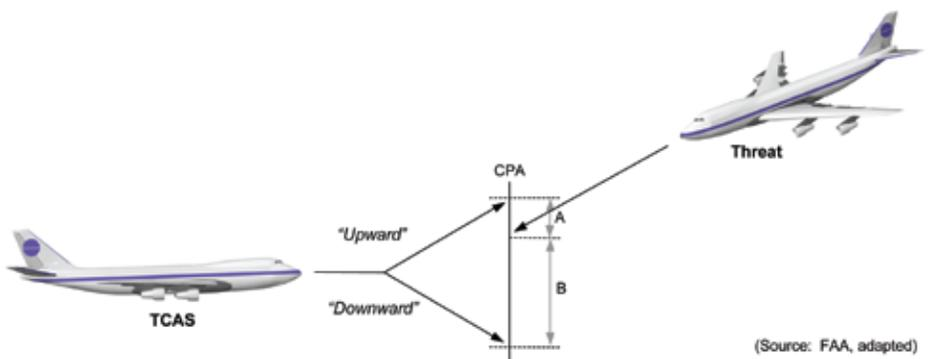
Today, TCAS is installed on all commercial aircraft with at least 30 passenger seats operating in the U.S. It receives and displays bearing and relative altitude information about all other aircraft within a 40-mile radius and provides alerts and its Resolution Advisory with respect to the aircraft that poses the greatest potential threat.
