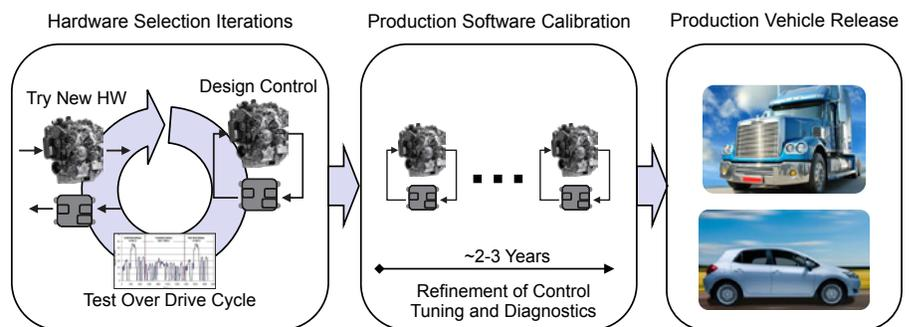
*Every step of the powertrain development process involves control design. Today's process typically requires a few years from requirements specification to engine certification.*
