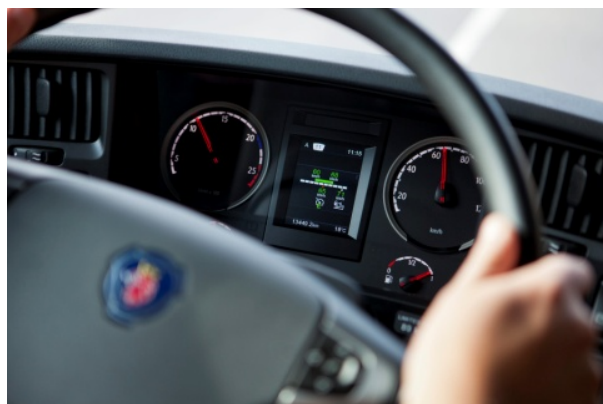
Scania Active Prediction in use. The cruise controller adjusts the vehicle speed within a range around the desired average speed in order to traverse hills more efficiently.
