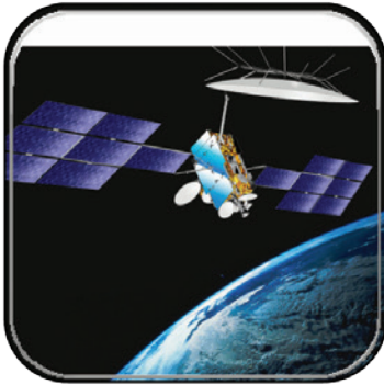
Artist's rendering of Eutelsat W2A satellite in orbit, based on the Spacebus 4000 C4 platform, with deployed solar arrays and 12-m-diameter antenna (Source: Thales Alenia Space)
