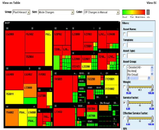
Color-coded graphics for plantwide CPM. The tiled rectangles refer to plant subsystems (e.g., units); the size of each rectangle can be proportional to energy consumption, alarm counts, or a user-defined property. Colors indicate the current assessment of each subsystem. (Source: BASF SE)
