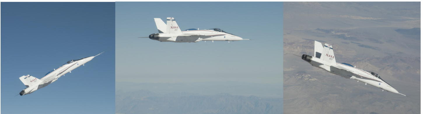
Photographs depicting the trajectory flown repeatedly by NASA's F/A-18 while testing the SLS AAC (2013, through a partnership among the NASA organizations MSFC, AFRC, NESC, and STMD-GCT)
