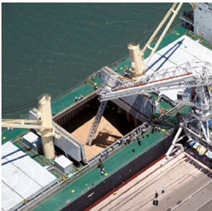
An unloader using its take-up point to dig into the grain in a hatch
