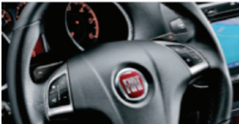
Shift buttons on the steering wheel of a FIAT Bravo (Source: www.fiat.it )
