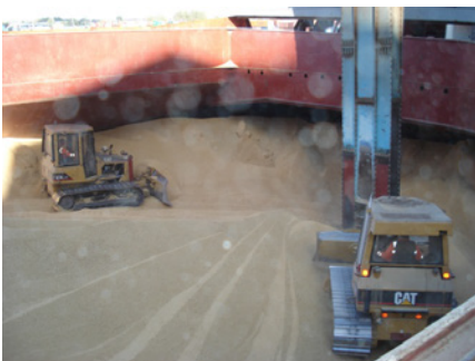
Two bulldozers feeding residual grain to the take-up point of an unloader in a hatch
