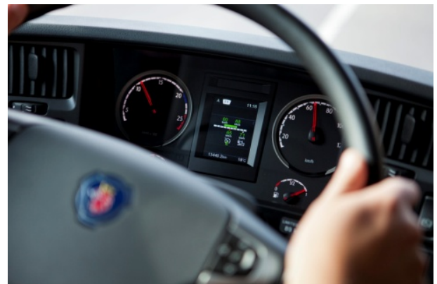
Scania Active Prediction in use. The cruise controller adjusts the vehicle speed within a range around the desired average speed in order to traverse hills more efficiently.
