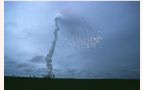
The Ariane 5 rocket had to be destroyed on its maiden flight because of a software bug (an arithmetic overflow). This incident renewed interest in formal verification and ultimately resulted in a success story for the technology.
