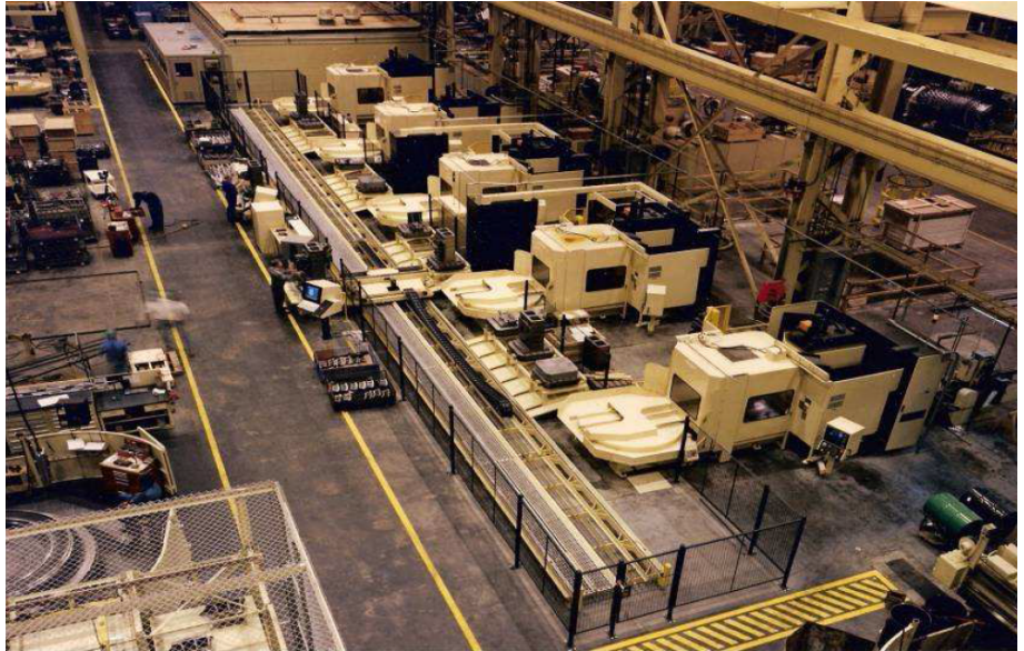
A flexible manufacturing system (Image courtesy of Cincinnati Milacron, Ohio)
