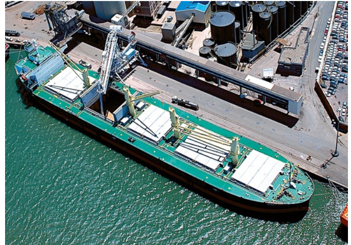
A five-hatch ship with a single unloader digging in hatch 4
