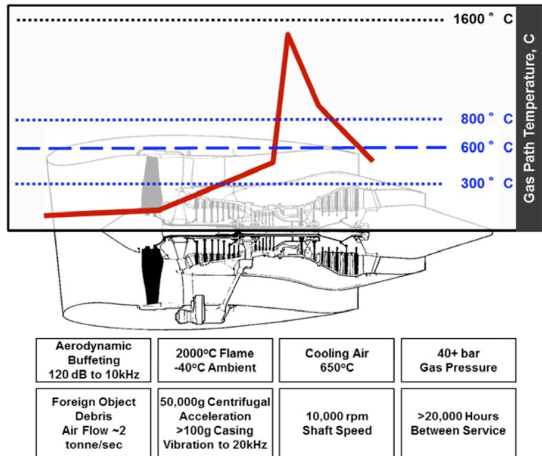
*Temperature extremes and vibration in the aero-engine environment are severe. The minimum temperature is due to ambient conditions at altitude, whereas the maximum temperature occurs in the combustor. Keeping the engine running under most fault conditions is essential.*
