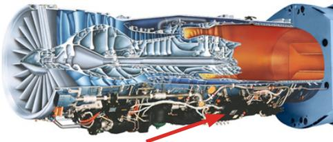
Currently, the ECU for military aircraft engines is core mounted, requiring fuel cooling. As the core becomes smaller and hotter, both the size and cooling requirements for the ECU become problematic.
