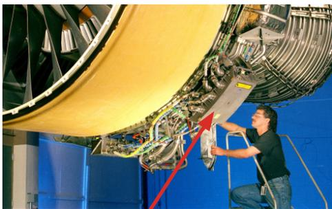
The present ECU for commercial aircraft engines is mounted on the cold fan casing. As the fan diameter increases, the push is to reduce the gap between the casing and the nacelle for weight and drag reduction. The size of the ECU becomes an issue.
