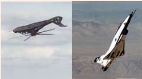
Left: RAH-66 Comanche demonstrating full flight envelope capability. Right: X-31 demonstrating high angle of attack maneuver. Sources: Boeing/Sikorsky and NASA
