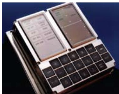
Apollo computer interface box used in the F-8C digital fly-by-wire program. Source: NASA
