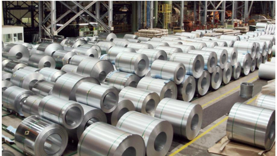
Galvanized steel coils ready to be shipped
