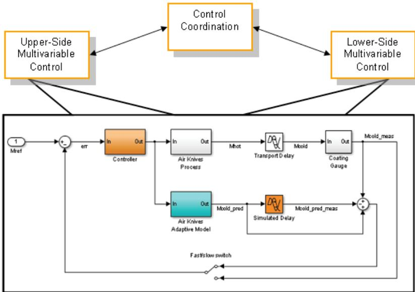
The coating control architecture. The air knife model is subject to online fine-tuning. The orange blocks are implemented in the regulatory control level, the cyan block in the supervisory control level. Only one side of the strip is represented here for simplicity.
