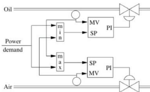
The PID controller is based on very simple ideas. As illustrated in the idealized formula below, the controller output is a combination of three terms:
