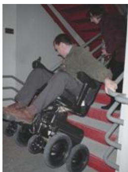
Stair climbing with the iBOT wheelchair (Source: D. Ding, R.A. Cooper, "Electric-powered wheelchairs—A review of current technology and insight into future directions," IEEE Control Systems Magazine , April, 2005)
