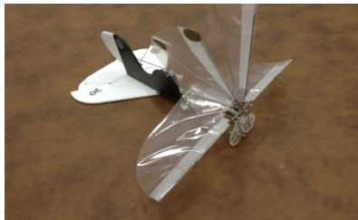
Conventional tail surfaces are used to control this flapping-wing MAV.
