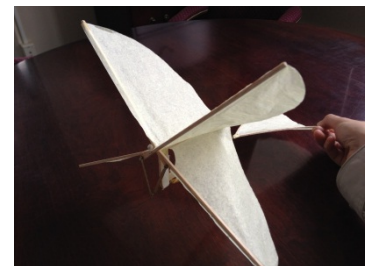
Balsa wood, tissue paper, wire, and rubber bands were used to create this ornithopter.
