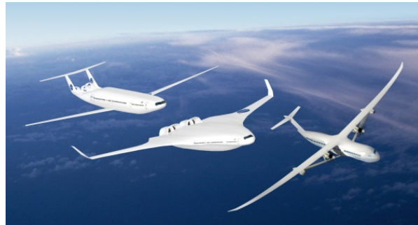
Aircraft design concepts for improved energy efficiency and environmental impact (Source: NASA)
